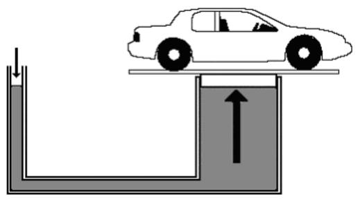
The mechanical advantage of the illustrated hydraulic lift here would be ...
