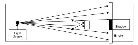
Light travels in straight lines until it strikes a surface. The type of surface will determine how the light will continue.
