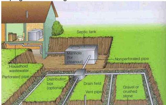
The remaining liquid waste is distributed through pipes with holes (perforated); the pipes lead into a drainage area containing gravel. Bacteria and other micro-organisms in the gravel and soil break down the organic waste and use it as a source of food energy. This system mimics the way in which decomposers normally recycle biodegradable wastes. The septic tank is periodically pumped out to prevent overflow.
