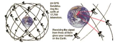
The three GPS satellites provide coordinated location information, which is transmitted to a GPS receiver (handheld) to indicate the person's exact position on the Earth.
