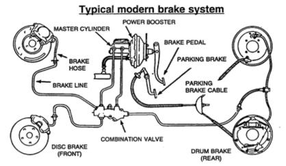
The brake fluid transfers the pressure from the brake pedal to the brake pads and the disc, which produces enough force to stop the car.
