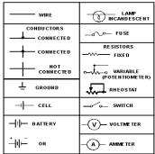
A drawing made with these symbols is called a *schematic* or schematic diagram.
