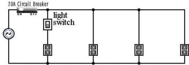
Typical 120V - 20A Parallel Circuit with 4 wallplugs - one of which is switched.
